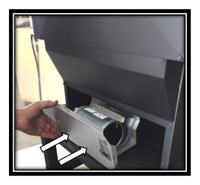
TILT FAN ASSEMBLY FORWARD AND SLIDE INTO THE OPENING LOCATED AT THE BACK OF THE UNIT. MAKE SURE THE FAN OUTLET IS FACING THE BACK OF THE APPLIANCE.
