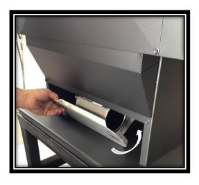
WHEN THE FAN ASEMBLY IS HALF WAY IN, START TILTING THE ASSEMBLY UPWARDS, UNTIL THE BASE PLATE IS AGAIN PARALLEL WITH THE BASE OF THE APPLIANCE.
