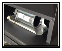
PLACE THE NUTS AND THE WASHERS SUPPLIED, THEN PULL THE FAN ASSEMBLY TOWARDS THE BACK OF THE APPLIANCE, AS FAR BACK AS ALLOWABLE, THEN TIGHTEN BOTH THE NUTS.
