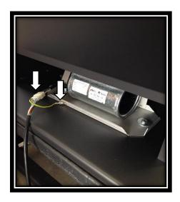
ATTACHED THE WIRING HARNESS AND THE GROUND CONNECTOR. TEST THE FAN AND MAKE SURE EVERYTHING IS WORKING PROPERLY. THE FAN IS READY FOR USE.
