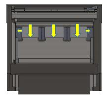
5. WHEN THE BAFFLE PLATES 1 AND 3 ARE IN POSITION, MOVE BAFFLE 2 FROM ATOP BAFFLE PLATE 1 INTO PLACE IN THE MIDDLE GAP, CENTRALISE AND PUSH TOWARDS THE BACK WALL. THIS WILL COMPLETE THE INSTALLATION
