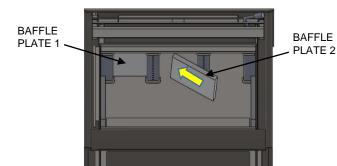
3. REPEAT STEP 2 PROCESS BUT THIS TIME MAKE SURE THE BAFFLE PLATE 2 SLIDES OVER BAFFLE PLATE 1.
