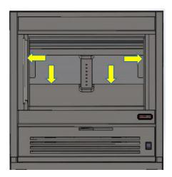
4. REPEAT THE PROCESS FOR THE OTHER SIDE. PUSH BOTH BAFFLE PLATES UNTIL IT IS AGAINST THE SIDE AND REAR WALLS.
