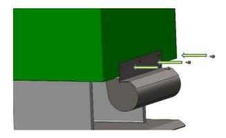
3. USE THE TEK SCREWS SUPPLIED AND FASTEN THE FAN ASSEMBLY TO THE APPLIANCE. A HEX HEAD SCREW DRIVE ON A DRILL IS REQUIRED.
