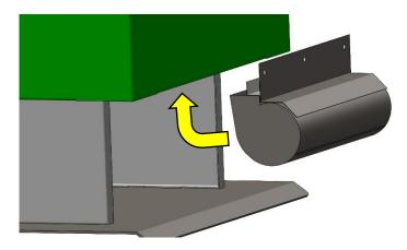
1. POSITION FAN ASSEMBLY ADJACENT TO THE REAR PANEL OF THE APPLIANCE, POSITION THE FAN IN BETWEEN THE CUT OUTS ON THE REAR PANEL. PUSH THE FAN ASSEMBLY AS HIGH AS ALLOWABLE.
