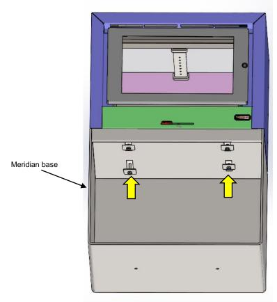
The bolts will need to be removed when the appliance is installed onto a meridian base. However, the same bolts must be used to fix appliance to the meridian base.
